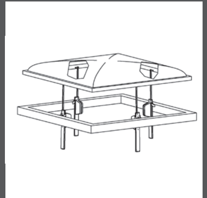
Installation on vertically opening domes
