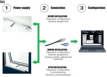
The UCS BMSline Configuration Software works on any computer with Windows XP and following versions
