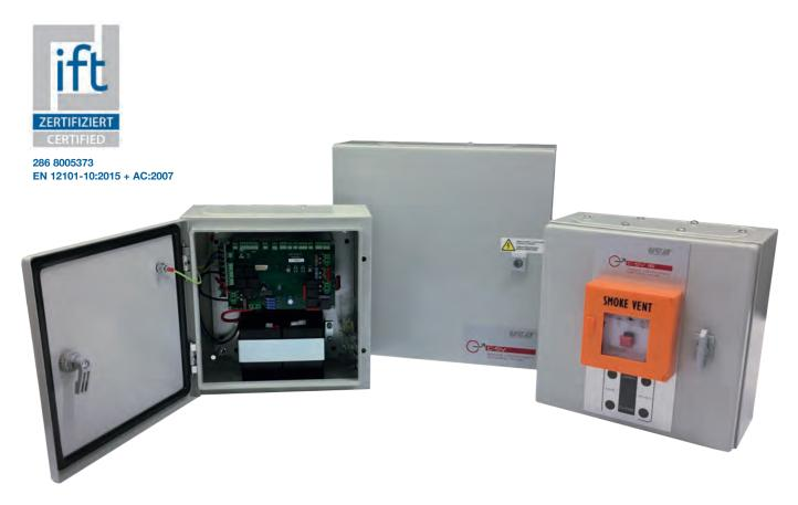
A very versatile range of smoke ventilation control panels, provided of back-up batteries: they operate 24 Vdc actuators for smoke and heat extraction in case of fire, and control the automation of single or multiple windows for natural ventilation even in a multy-storey building.
